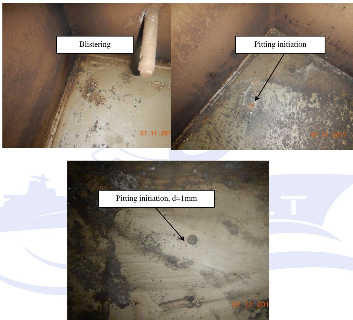
Figure 4 Initiation of pitting corrosion.
