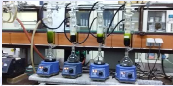
Figure 5. Soxhlet apparatus to extract algal oil with chemical solvent (hexane)
