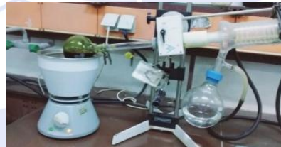
Figure 6. Drying algal extracted oil using rotary evaporator.
