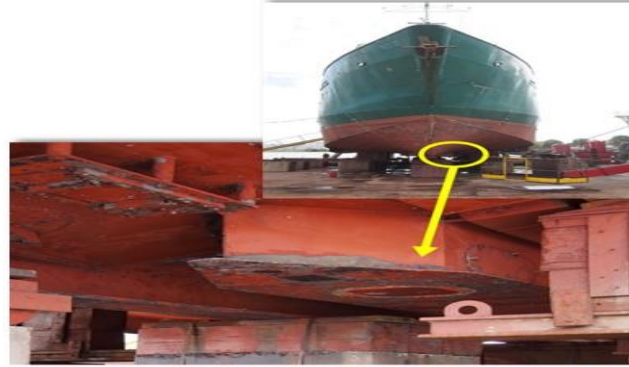
Figure 1. The EK60 transducer on the hull of the RV Weatherbird II. (Photo courtesy of Matt Hommeyer).
