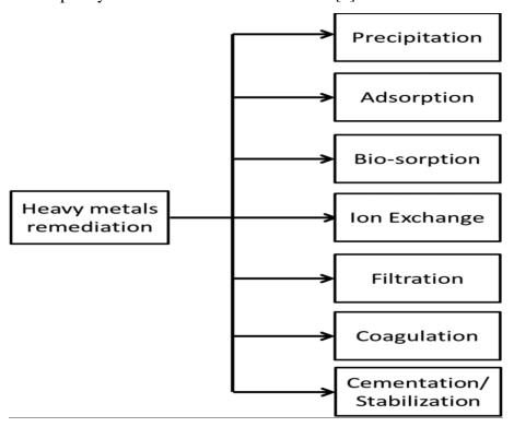
Figure 1. Mechanisms of heavy metals removal [20].
